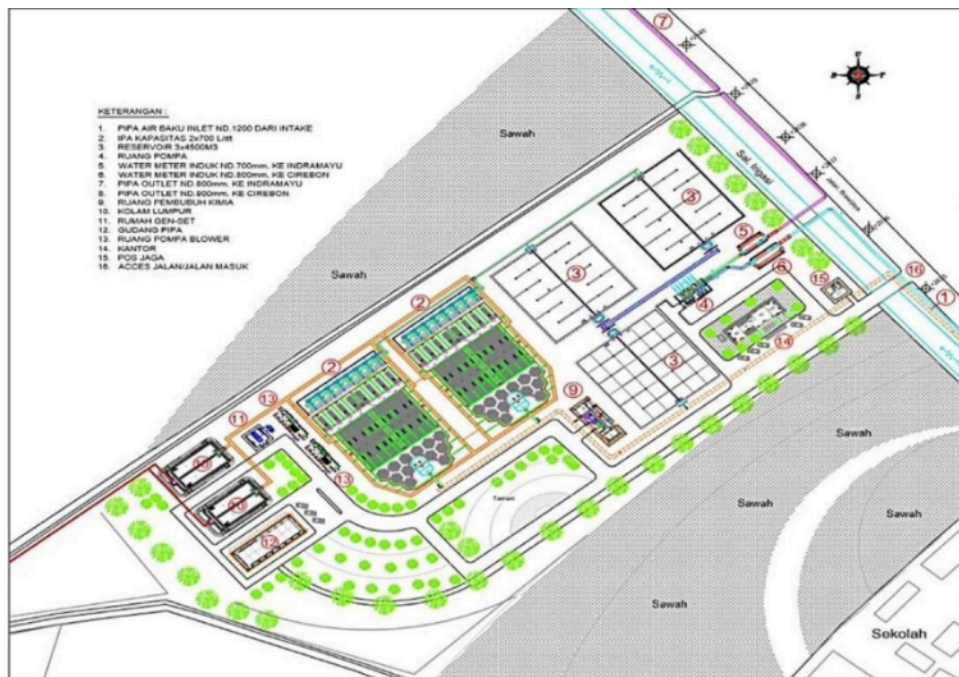
Picture 1 – Layout of Jatigede Water Supply System
